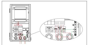
Use the screwdriver to remove the nut with position numbers 4 and 6 in the contactor, and then insert EPS-L1, EPS-L2 wire into the port of contactor (4&6) through the cable nut and tighten them with screwdriver. Use a screwdriver to lock the ground wire on the earth
