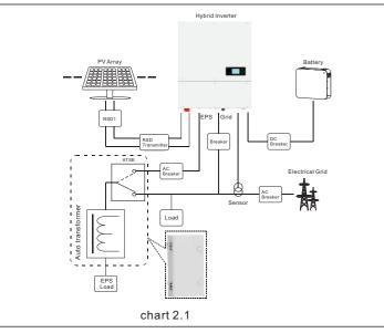
As shown in chart 2.1, the input side of ATS-US is connected with EPS output of hybrid inverter and grid, the output side is connected with critical load stated as EPS load. EPS Load is set default to connect with Grid power.If Grid is lost, EPS Load will turn the switch to EPS output of hybrid inverter. And there is a transformer in ATS-US, it can transform 240V to 120/240V split phase to provide the power to critical load.
