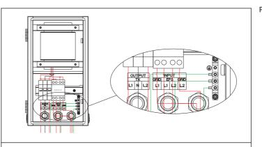
Use the screwdriver to remove the nut on the terminal strip, and the red 10AWG short wire ends were inserted into the port L1 and L2, The Black 10AWG short wire ends were inserted into the port N. Use a screwdriver to lock the ground wire on the earth bus bar.
