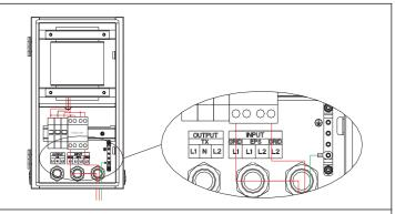
Use the screwdriver to remove the nut with position numbers R2 and R8 in the contactor, and then insert GRID-L1, GRID-L2 wire into the port of contactor (R2&R8) through the cable nut and tighten them with screwdriver. Use a screwdriver to lock the ground wire on the earth bus bar.
