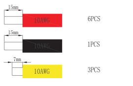
3. There are two types wire need to be machining, please check ref to 9.1 wired diagram. The follow two type wires are show as below (type1 is used to power line connection, type2 is used to ground connection):
