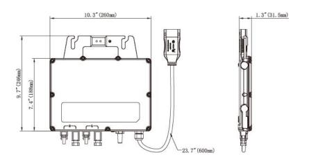
YC600B was designed to accommodate today's high output PV panels, offer enhanced capability and meet the latest grid compliance standards. Offering an unprecedented 300VA peak output power per channel, the YC600B works with 60 and 72-cell PV modules and offers dual, independent MPPT per panel. The YC600B also operates within a wider MPPT voltage range than competing brands for a greater energy harvest.
