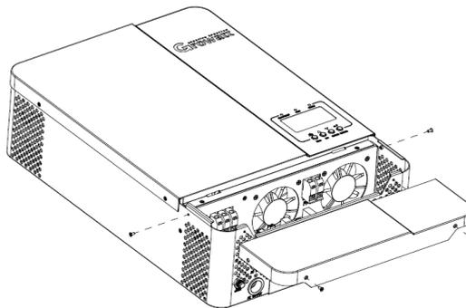
**Step 2:** Remove WiFi/GPRS communication board and CAN/RS485 communication board by unscrewing screws as below chart.
