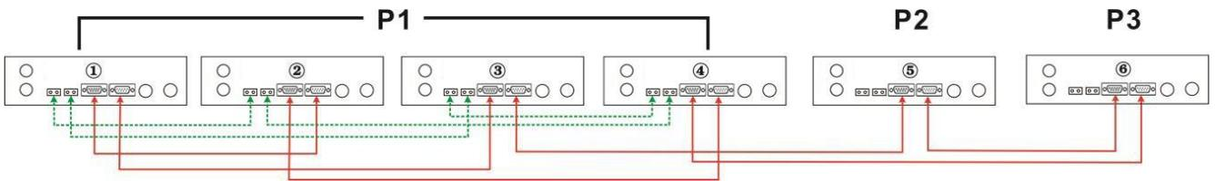
**WARNING:** Do not connect the current sharing cable between the inverters which are in different phases.
