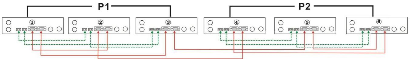
**WARNING:** Do not connect the current sharing cable between the inverters which are in different phases.
