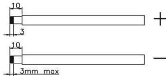
2. Check correct polarity of connection cable from PV modules and PV input connectors. Then, connect positive pole (+) of connection cable to positive pole (+) of PV input connector. Connect negative pole (-) of connection cable to negative pole (-) of PV input connector.
