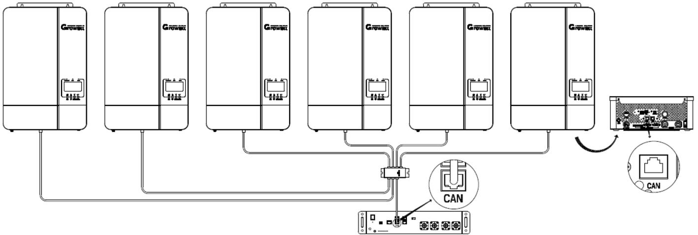
**Note:** The above diagrams described the parallel system communicate with lithium battery in CAN communication type, and it is the same to the RS485 communication type. Only need to change to "RS485" port if you use RS485 for communication.
